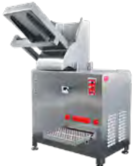
GS 510 Block cross-section 500 x 300 mm Processing temperature > -15°C Max. throughput 4000 kg/h
